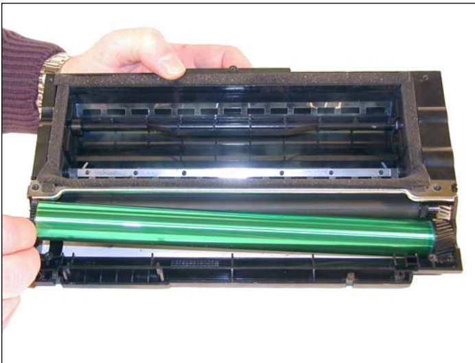
19. Install the new drum in place.
