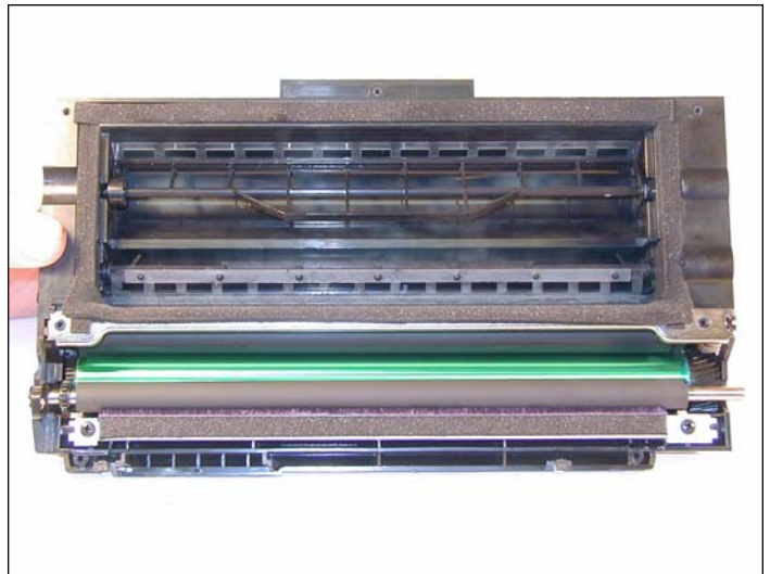
22. Install the PCR. Make sure that the PCR gear is on the correct side and that the shaft is in the PCR holder.
